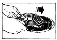
Hold the surface unit as level as possible with the terminal just started into the receptacle. Push the surface unit terminal into the receptacle.
