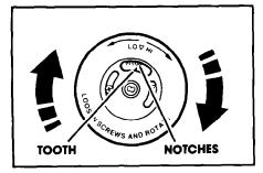
**4.** To raise the temperature, move the tooth a notch closer to HI. Each notch equals about 10°F (5°C).
