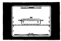
4. Put food in the oven. During baking, the elements will turn on and off to keep the oven temperature at the setting. The Oven HEATING Indicator Light will turn on and off with the elements.
