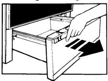
Empty drawer of any pots and pans before removing drawer. Pull drawer straight out to the first stop. Lift front and pull out to the second stop.
