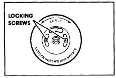
2. Loosen the locking screws inside the control knob. Note the position of the notches.
