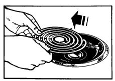
**3.** Pull the surface unit straight away trom the receptacle.
