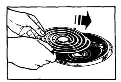
Hold the surface unit as level as possible with the terminal just started into the receptacle. Push the surface unit terminal into the receptacle.
