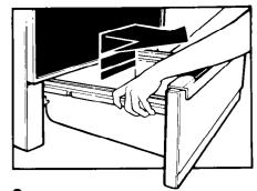
2. Lift back slightly and slide drawer all the way out.
