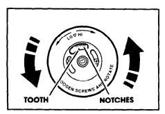
To lower the temperature, move the tooth a notch closer to LO. Each notch equals about 10°F (5°C).
