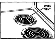
The vent is needed for air circulation. **Do not block the vent.** Poor baking can result.
