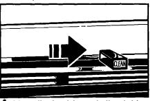
Move the Lock Lever to the right – the Clean position. The Oven HEATING and ON Indicator Lights will come on.
