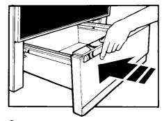
Lift drawer front and push in until metal stops on drawer slide rails clear white stops on drawer guides. Lift drawer front again to clear second stop and slide drawer closed.
