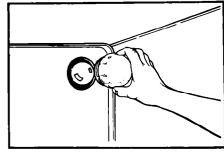
Remove the glass bulb cover in the back of the oven by screwing it out counterclockwise.
