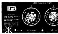
5. The Oven LOCKED Indicator Light comes on when the oven temperature exceeds normal baking temperatures. The Lock Lever must not be moved and the door can't be opened when the Oven LOCKED Indicator Light is on.
