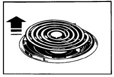
2. Lift the edge of the unit, opposite the receptacle, just enough to clear the element hold down clip, reflector bowl and trim ring.
