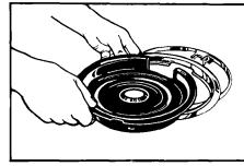
2. Line up openings in the reflector bowl and notches in the trim ring with the surface unit receptacle and the element hold down clip.
